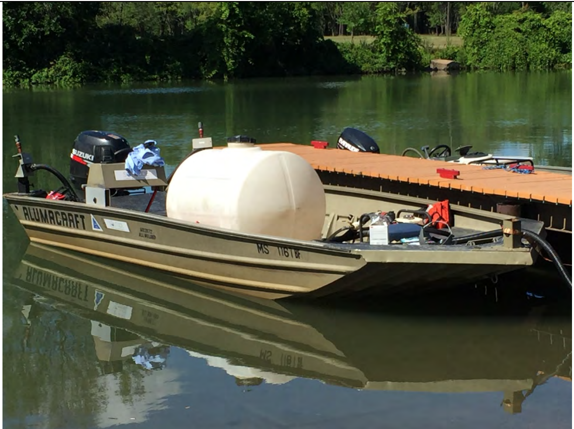
Date: 07/26/2016 Direction of View: West from North shore of creek Subject: Application boat set-up Description: Endothall was placed in the tank and dispensed into the creek through PVC pipes on back of boat.
